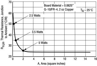
Figure 16. Thermal Resistance versus Drain Pad Area for the D<sup>2</sup>PAK Package (Typical)
