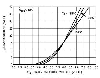
**Figure 2. Transfer Characteristics**
