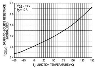
Figure 5. On–Resistance Variation with Temperature
