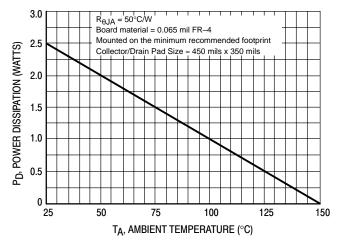
Figure 15. D<sup>2</sup>PAK Power Derating Curve
