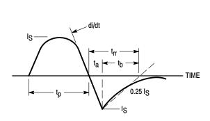
Figure 14. Diode Reverse Recovery Waveform
