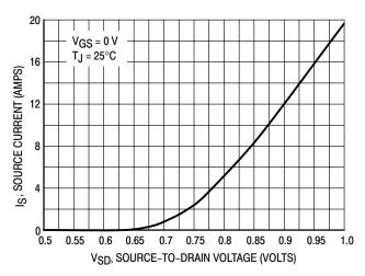
Figure 10. Diode Forward Voltage versus Current
