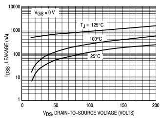
Figure 6. Drain-To-Source Leakage Current versus Voltage
