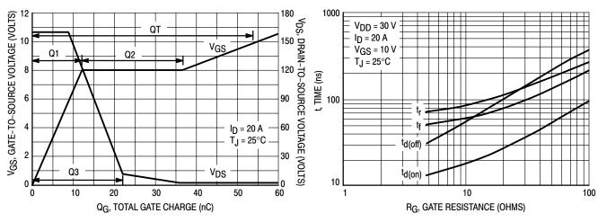
Figure 8. Gate-To-Source and Drain-To-Source Voltage versus Total Charge
